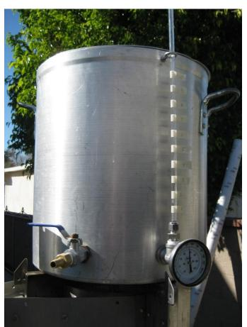
I added the sight glass and thermometer when I switched to the three tier stand, so I could see the water level and temperature without having to climb up a ladder. The mash tun is the common round, orange cooler. It has a metal domed screen as a false bottom, and a high temperature hose with a simple clamp for flow control. The boil kettle is a new addition to the system.
