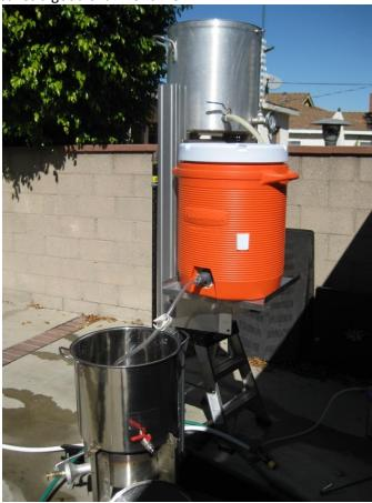
With these additions and changes, I've cut my 6-8 hour brew day down to about 4 hours from start to finish, including setup and cleanup. The biggest time savings were in the switch to a three tier, gravity fed system, and the use of an immersion chiller. Both changes save a large amount of cleaning and sanitation time. Future plans include the motorized wort stirrer mentioned
