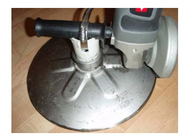
Make sure you get a cut off wheel; they are thinner than the one that it comes with the grinder. Make a few passes with the grinder; don't cut all the way through on the first pass. You'll notice that the edges will be rough, I took some 60 grit sand paper and smoothed out the edges in a few minutes, both the top and bottom edge.
