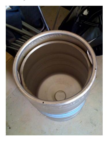
Step 2: Now it's time to drill the holes for the bulkhead and sight glass fittings. You can use a weld less bulkhead
