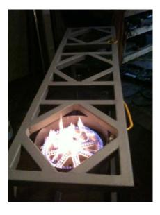
I bought the gas manifold from Home Depot and used water heater gas lines from HD as well. Added 2 March pumps to move the liquid around and I'm all set. Painted it with high temp header paint from an auto parts store.
