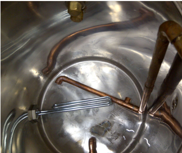
Figure 4: Kettle whirlpool arm, heating element, drain siphon and temperature probe
