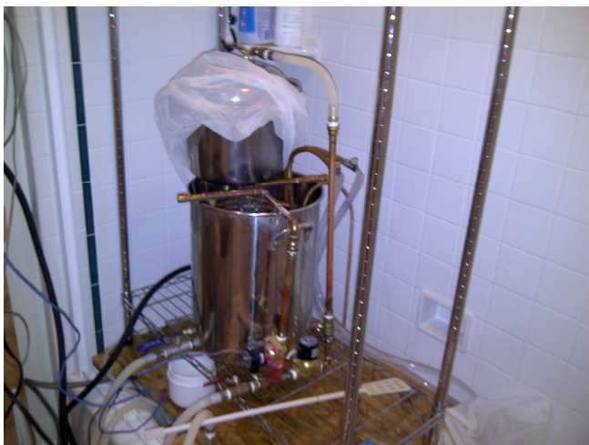
Figure 6: RIMS with gravity mashtun above kettle
