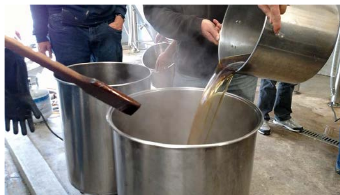
At the same time, the recipe's sugar was inverted by heating to 150F with water, acid and invertase enzyme then boiled to drive off the water and become caramel. In a second pot, 15 gal of first runnings wort was also caramelized and both were added to the brewery kettle. The inverting and caramelizing steps took 20 pounds of propane. If more was available, a longer boil would have intensified the caramel flavors and darkened the beer.
