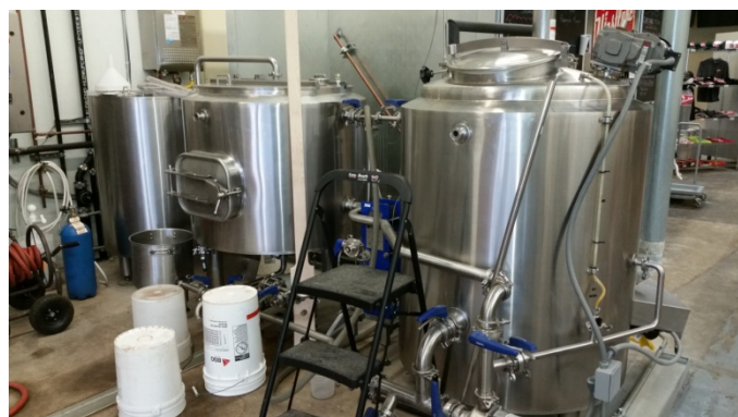
The direct fired brewery has three vessels on a small footprint. The hot liquor tank is on the left, the lauter tun is in the middle and the combination mash tun/kettle is on the right. Westlake Village tap water was filtered through activated carbon and its alkalinity was raised with a mineral addition. Mash water was heated in the HLT, pumped by a multi-tasking portable pump to the mash tun where it was manually mixed with the grist at 120F, held for 15 min, heated to 150F, held for 45 min and finally mashed out at 168F.
